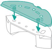
3 Slide the straight side of the washable mop pad in the correct slot of the mop pad holder and attach the washable mop pad to the velcro material of the mop pad holder.
