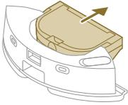
2 Open the lid of the dust bin and let the dirt out of the dust bin.
