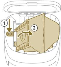
2 Press the release button and push the bag holder to the side.
