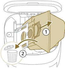
3 Remove and dispose the dust bag.
