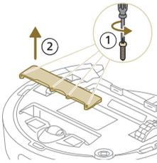
3 Undo the screws of the battery compartment lid and remove the lid.
