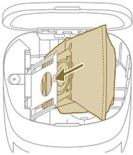
4 Slide the cardboard piece of the dust bag onto the bag holder.
