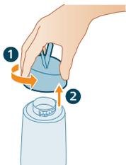
2 Unscrew and remove the water tank cap.
