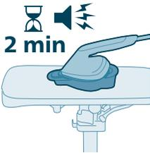
**15** During the Calc-Clean process, you hear short beeps and a pumping sound. Wait approximately 2 minutes for the appliance to complete the process.
