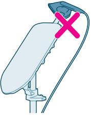
**10** Do not dock the iron in a tilted position. This can cause the iron to drop from the dock.
