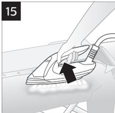
**Note: For best result on tough fabrics such as cotton, linen and denim, keep the steam trigger pressed continuously when you move the iron over the fabric (Fig. 15). Then move the iron over the same area a few more times without steam to dry the fabric.**
