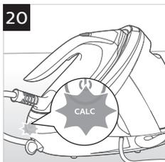
**It is very important to use the EASY DE-CALC function as soon as the EASY DE-CALC light starts to flash (Fig. 20) and the appliance beeps continuously.**
