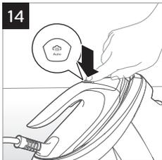
You can control the amount of steam manually during ironing by turning off the intelligent automatic steam mode .
